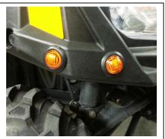
6. Repeat steps 3-5 to install the rear signals for the machine. Remember that the polarity on LED lights is critical. Please refer to the Wire Harness Diagram included with the harness packaging to ensure you get the positive and negative wires correctly in place.
