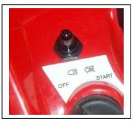
12. To mount the horn switch, drill a  $\frac{1}{2}$ " hole in the desired area in the dash. Install the switch through the hole and put the sealed rubber nut on.
