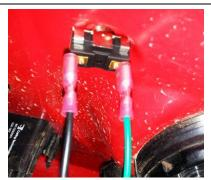
14. To mount the indicator lights, drill a 5/16" hole on both the left and right side of the turn signal switch. Feed the wires of each indicator light through the hole and thread on the nut to secure the light. Plug in the lights, but make sure the indicators are connected to the correct wires on the harness (again, refer to the wire diagram).
