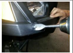
5. To mount the signal, first remove the rubber grommet from the light. Push the grommet into the hole until it is seated correctly into the hole. Feed the wires of the light into the new hole you drilled. Notice the direction on the lens; make sure the "Top" is at the upper point of the light. <u>Plug the black wire from the signal into the positive wire on the harness and the white signal wire into the ground signal wire.</u>
