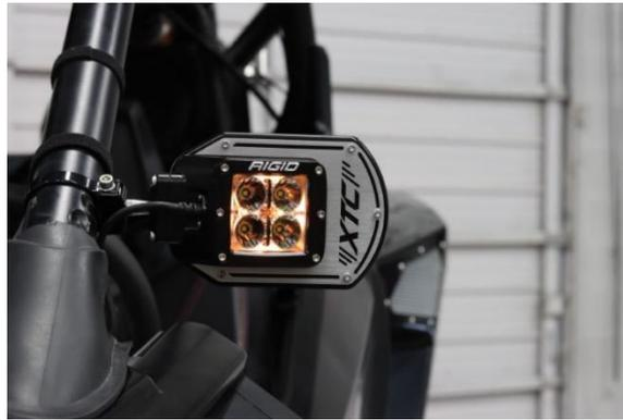
3. Install the wiring harness. The kit comes with a standard 36" power cable, optional Plug & Play power cables can be purchased at [www.xtcpowerproducts.com](http://www.xtcpowerproducts.com).
