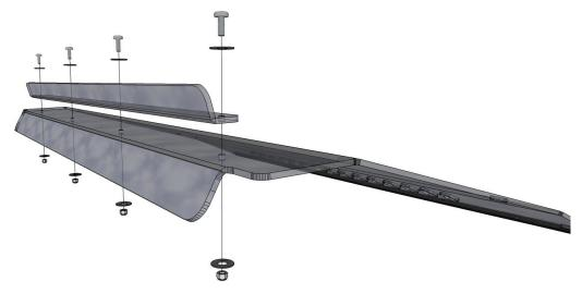
8. If you are using this windshield with a Over Armour Cab enclosure then you will use the Top Brace to sandwich the cab material and seal off the inside from the wind. The diagram below shows how it will work. If you aren't using one of Over Armour Cab Enclosure you may opt not to use the Top Brace or install it for added strength.
