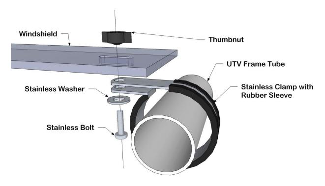
7. Now you can install the top brace if you want. If you do not have a Mammoth Designs Cab enclosure to work with this windshield, the top brace is not needed but can be installed for extra strength. Below is a diagram showing how the brace is to be installed.
