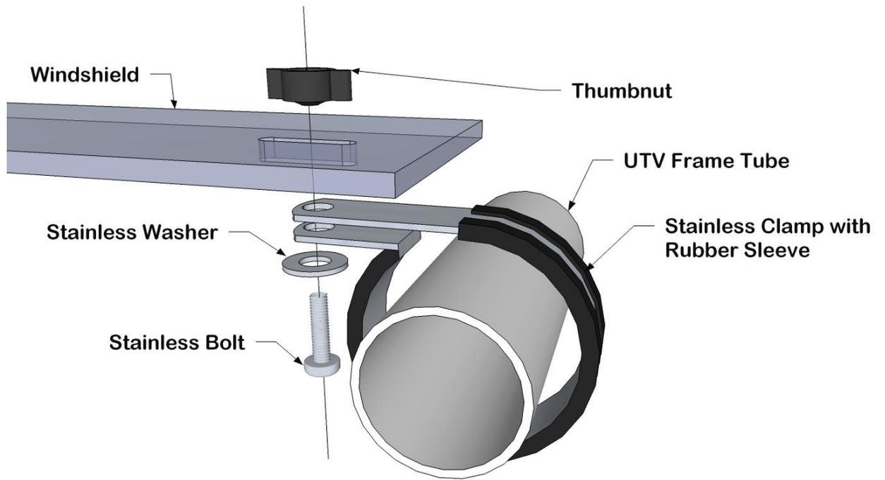
7. Now you can install the top brace if you want. If you do not have a Mammoth Designs Cab enclosure to work with this windshield, the top brace is not needed but can be installed for extra strength. Below is a diagram showing how the brace is to be installed.
