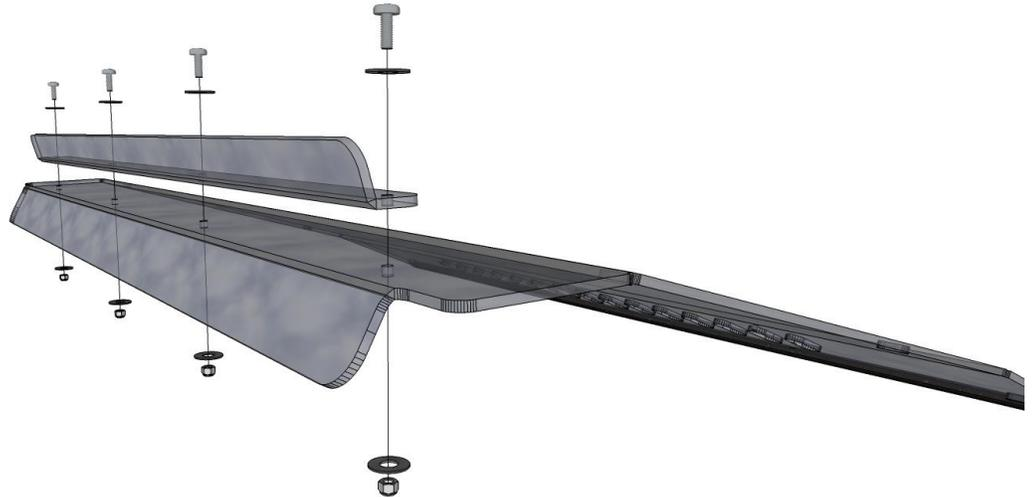
8. If you are using this windshield with a Over Armour Cab enclosure then you will use the Top Brace to sandwich the cab material and seal off the inside from the wind. The diagram below shows how it will work. If you aren't using one of Over Armour Cab Enclosure you may opt not to use the Top Brace or install it for added strength.
