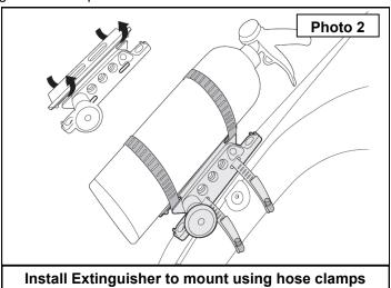
3. Note there are 2 holes for a flat mounting surface if desired. Hardware not included. See Photo 3.
