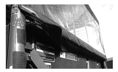
4. Now pull the rear window up and attach it to the top bar across the back of the roll cage. The top and sides of the rear window has double-sided Velcro sewn along the edges. At each of these strips you will place a 3" adhesive Velcro strip on the inside of the bar to hold the double-sided Velcro in place. The diagram below shows how to place the Velcro.
