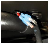
Figure 16: Harness to Light Cable Connection
