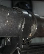
Figure 9: ROPS Loop Notch Detail
