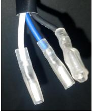
Figure 19: Switch Connectors (stock switch removed)
