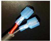
Figure 13: Spade Connectors on Light Bar Cable
