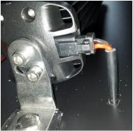
Figure 12: Routing Cable Through Roof
