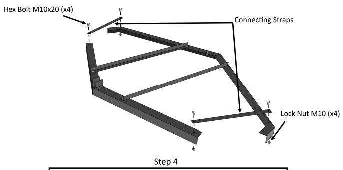
Connect the Front Angle Assembly to the Rear Angle Assembly with the two Connecting Straps using four M10x20 Hex Bolts, and four M10 Lock Nuts.
