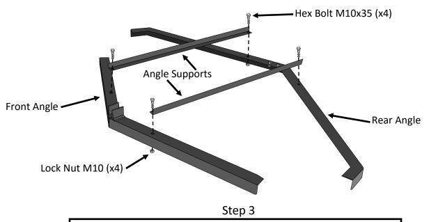
Connect the Front Angle Assembly to the Rear Angle Assembly with the two Angle Supports using four M10x20 Hex Bolts and four M10 Lock Nuts.
